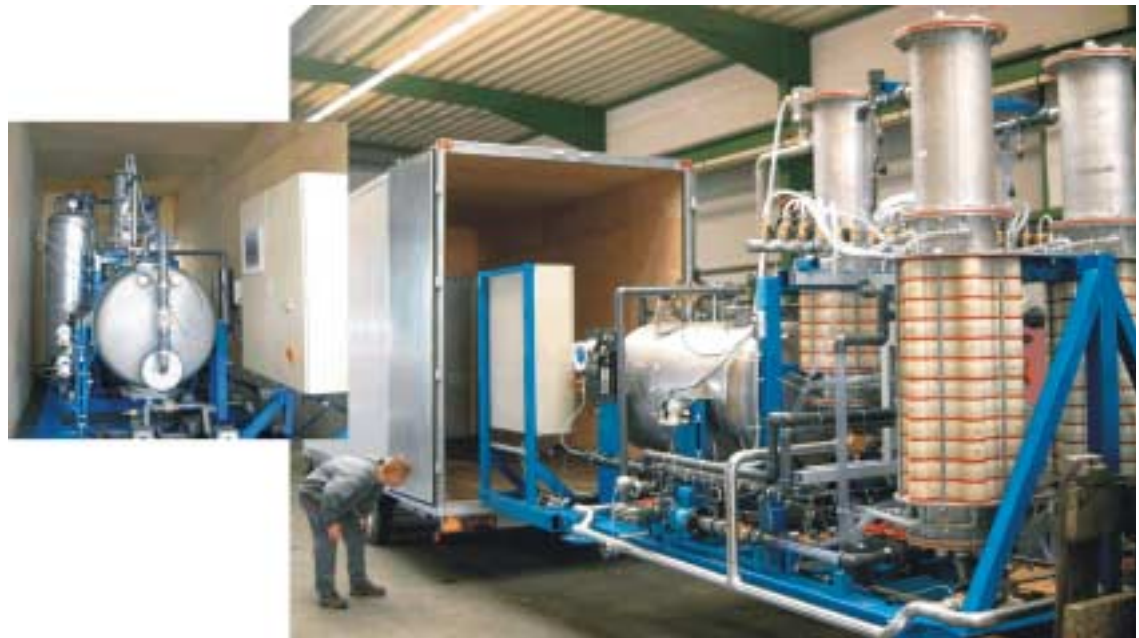
Mobile Drinking Water Treatment Plant using Kontaktor®-membranes for Micro and Ultra-filtration of surface water
